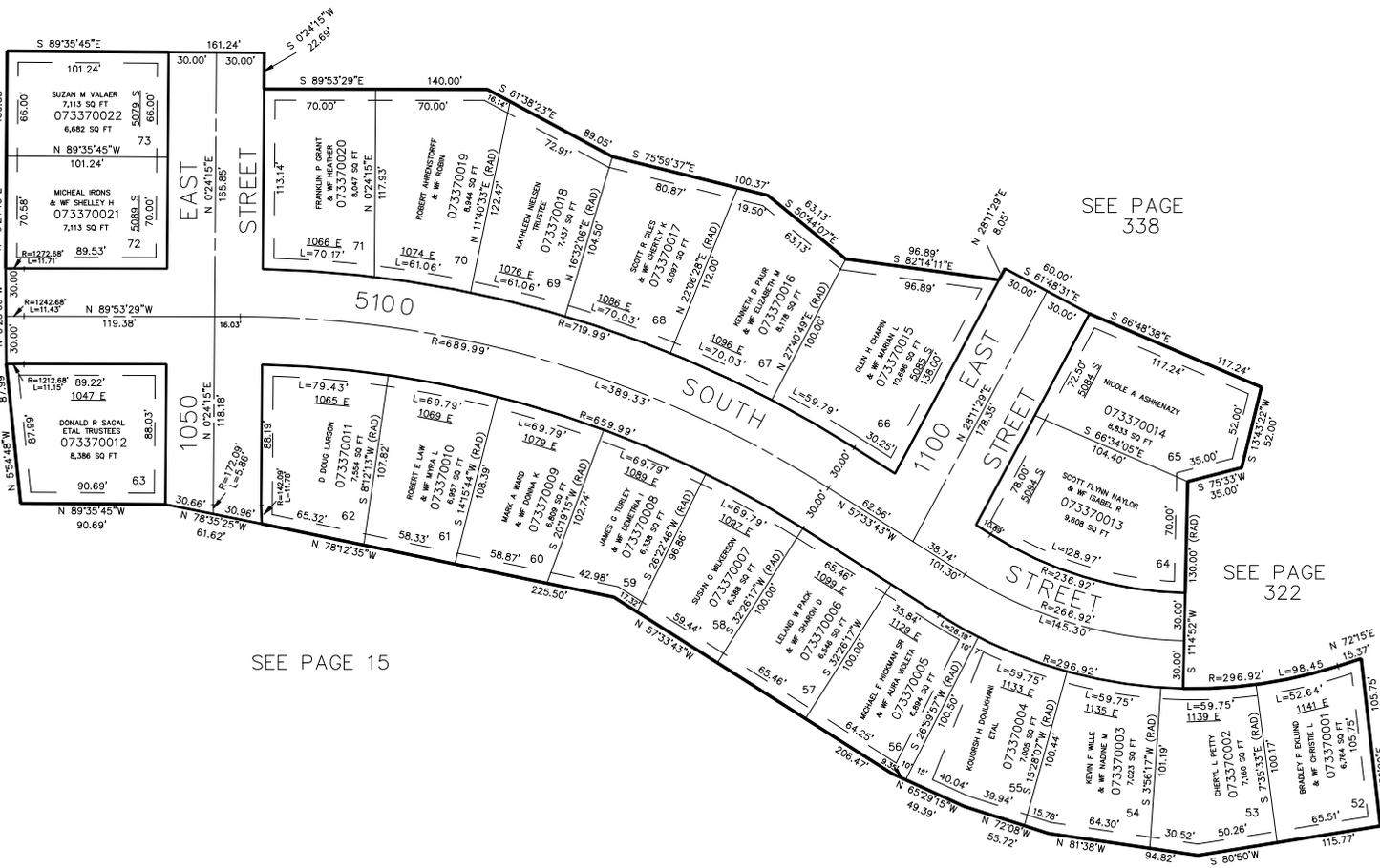
7' UTILITY AND DRAINAGE EASEMENTS EACH SIDE OF PROPERTY LINE, AS INDICATED BY DASHED LINES, UNLESS OTHERWISE SHOWN.
